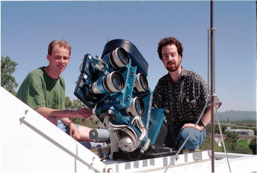
Figure 3.4. The original ROTSE (Robotic Optical Transient Search Experiment) telescope photographed with Jim Wren and Robert Kehoe, two of its operators in 1998. The telescope consists of four 200-millimeter telefocal lenses attached to CCD cameras and on a computer-controlled mount.
