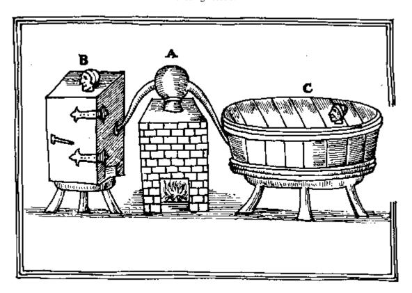
A. Signifies a hot still with two pipes going into two wooden vessels. In this still you may put either herbs, spices, with water or with spirits, and distill them, by which means they that are in the vessels will presently be forced into a
