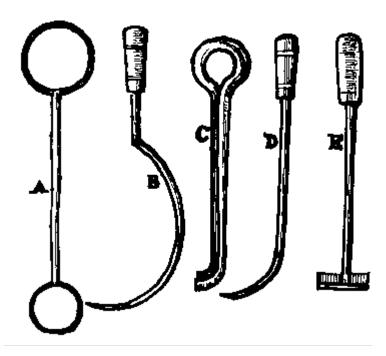
A. Signifies an iron rod with two rings at the ends thereof, which must be heated red hot and applied to that part of the glass which you would break off. When you have held it there so long until the glass becomes very hot, then take it off and drop some cold water where you would have it break off, and it will presently crack in sunder. These rings
