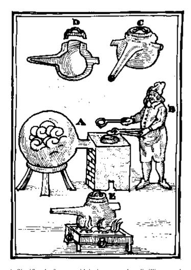
A. Signifies the furnace with its iron or earthen distilling vessel walled in, to which a very large recipient is joined. B. The distiller who with his left hand takes off the cover and with his right casts in his prepared matter with an iron
