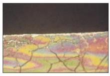
**Figure 5 -** 9ct gold-silver alloy treated 15 minutes at 600°C in alum paste. x250
