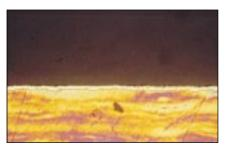
**Figure 11 -** 9ct gold-silver-copper alloy heated 2h in a boiling solution of alum. x400
