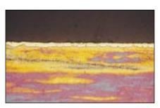
**Figure 12 -** 9ct gold-silver-copper alloy given 9 cycles of torch heating in alum paste and brick dust. x400
