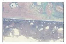
Figure 3 - Vicus disc showing gold flecks in corrosion products. x200
