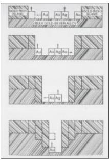
**Figure 14** - Corrosion and diffusion reordering model by selective dissolution. After Forty et al (15,16)
