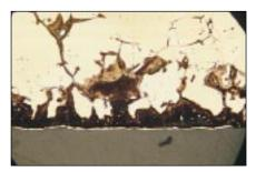
Figure 2 - Cross-section of Vicus disc showing depletion gilded layer. x200
